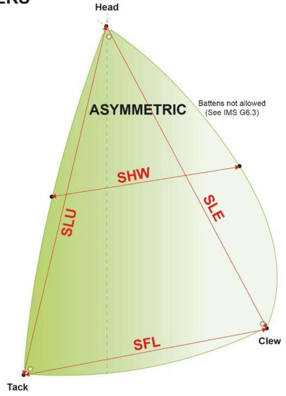
G6.1 half width of any spinnaker shall be 75% or more of the foot length. If not, the sail shall be measured as a headsail
